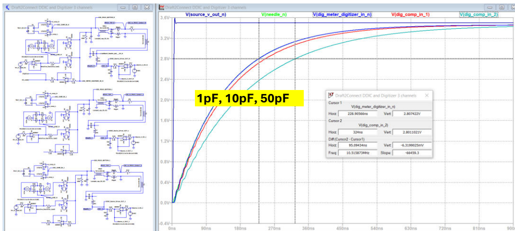
Fig 10. Response of DDIC Source 3.5V step signal with 10pF, 10pF, and 50pF Dig-Channel + Loadboard capacitance
