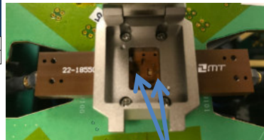
Dual Tx/Rx Patch antenna in contactor
