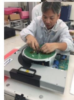
Dual Tx/Rx Patch antenna in contactor
