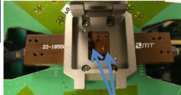
Dual Tx/Rx Patch antenna in contactor
