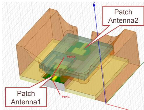
Modeled OTA Solution with Patch Antenna in Contactor
