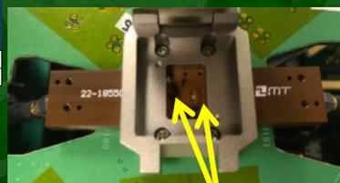
Dual Tx/Rx Patch antenna in contactor
