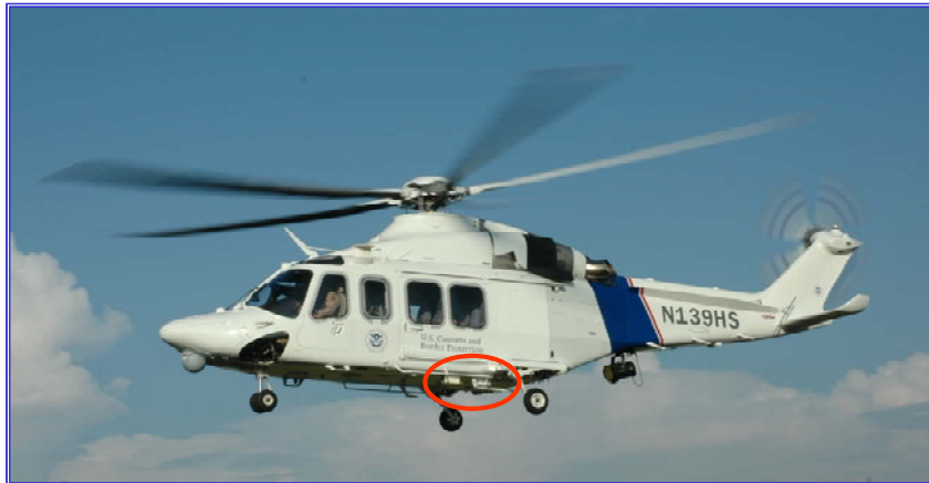
US Customs Helicopter with BMS Microwave Down-Link
